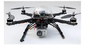
Drones need multiple horizontal rotors in order to achieve the level of control necessary for the unmanned aerial vehicle to be self-reliant. The rotors generate a lift force as they rotate, with a faster rotation generating more lift.
